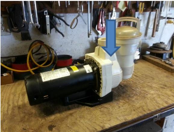
**2 Remove the bolts through the plastic and the pump can be separated.**
